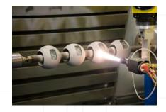
ValvTechnologies has developed a proprietary compressive spray technique which results in significantly higher bond strength and will better be able to control the quality of our process, reduce costs and improve lead times providing our customers with faster turnaround, a longer-lasting product, cost savings and higher bond strengths in the form of compressive coatings.
